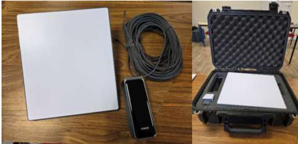
Figure 7: Mini-Starlink (with 2 batteries)
